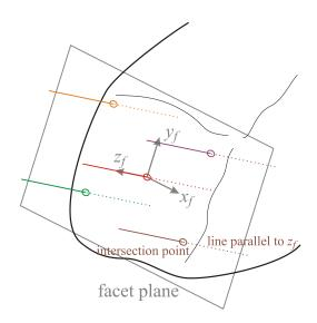
Fig. 3. Schematic illustration of the method applied to analyse the formation and growth of grain boundary facets.
