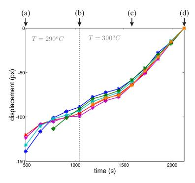
Fig. 4. Displacement of grain boundary segments forming a facet with reference to their final position along several parallel spatial lines as indicated in Fig. 2. The timings of the snapshots of Fig. 2 are indicated on top of the figure.
