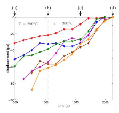
Fig. 6. Displacement of the grain boundary with reference to its final position along a set of parallel spatial lines indicated in Fig. 5. The timings of the snapshots of Fig. 5 are indicated on top of the figure.
