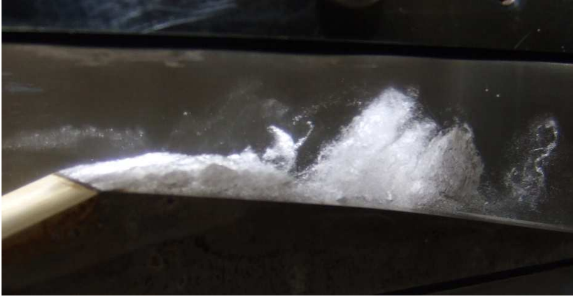
Figure 13. Photograph of the cavity, 8° Venturi
