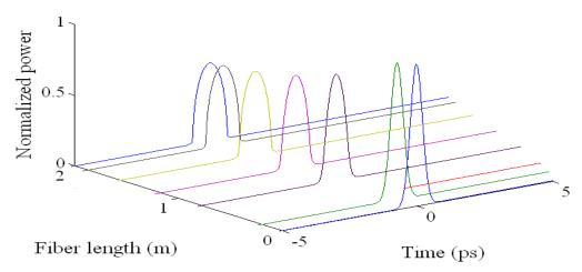
Fig. 6(b). Evolution of an input Gaussian pulse to a parabolic pulse with propagation in a lossless 2 meter long proposed tapered CBLF.
