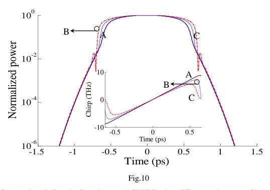
Fig. 10 Generated parabolic pulse from the tapered CBLF for three different peak powers of input pulse, 600 W peak power (solid curve 'A'), 800W peak power (dotted curve 'B'), and 1000W peak power (dash-dotted curve 'C'); Inset: Chirp variations over the pulse duration corresponding to the above three respective input conditions.
