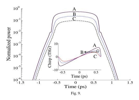
Fig. 9. Generated parabolic pulse from the tapered CBLF for three different cases, namely without loss (solid curve 'A'), 1dB loss (dotted curve 'B'), and 2dB loss (dash-dotted curve 'C'); Inset: Chirp variations over the pulse duration corresponding to the above three respective configurations.
