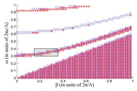
Fig. 2(a). Band diagram plotted here for two different cladding periods; first one:  $d_1$ = 0.44 µm,  $d_2$ = 0.85 µm ('blue circles (o)'), second one:  $d_1$ = 0.66 µm,  $d_2$ = 0.85 µm ('red stars (\*)'). In both the cases, we have assumed the periodicity is invariant over infinite cladding.
