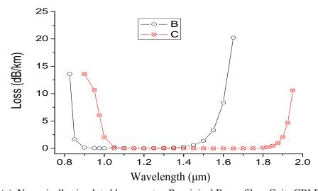
Fig. 3(a). Numerically simulated loss spectra, B: original Bragg fiber, C: its CBLF counterpart.
