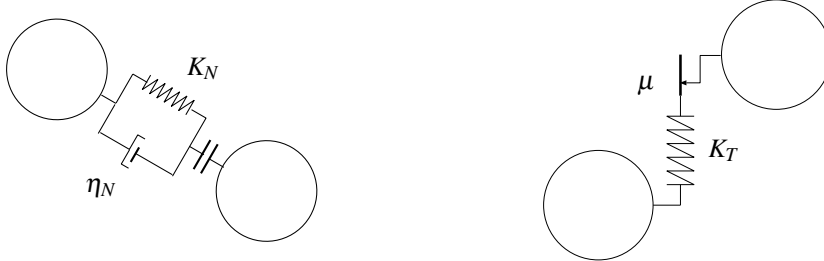
FIGURE 2. Normal (left) and tangential (right) contact behavior in 2D disk samples, as schematized with rheological elements: springs with stiffness constants K_N , K_T , dashpot with damping constant \eta_N , plastic slider with threshold related to normal force by coefficient \mu .
