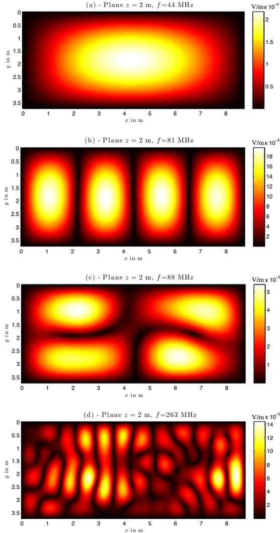
Fig. 4.  $E_z$  component of the electric field (linear values) in the plane  $z = 2$  m at different frequencies. Various cavity modes: (a)  $TE_{110}$ , (b)  $TE_{410}$ , (c)  $TE_{220}$  and a combination of different cavity modes (d).
