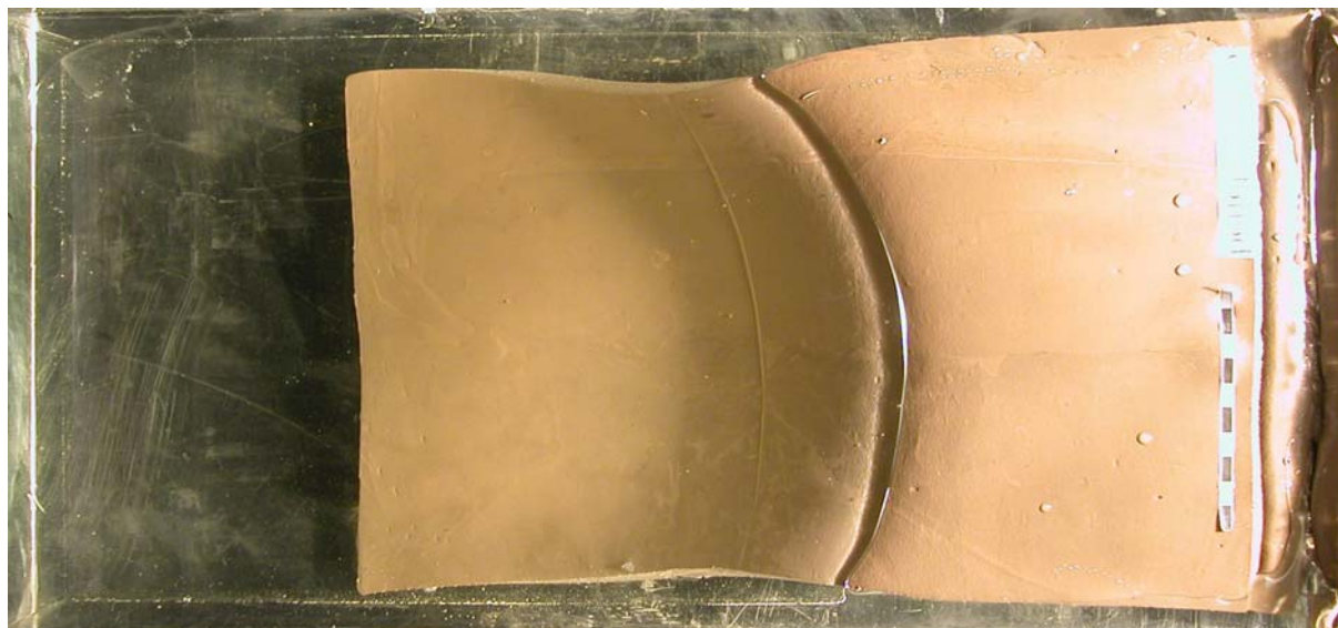
Fig. 15: Surface view of the laboratory model at the time 19' 15" illustrating the 3D effects. The brighter part of the plate on the right is still at the surface, the subducted part lies left of the arcuate trench.
