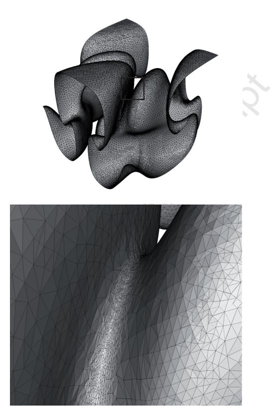
Figure 6: Geometry and triangulation of an originally flat surface deformed by a prescribed periodic and incompressible velocity field. The bottom panel is a close-up of a region (indicated on the top panel) where the surface curvature has become very large.
