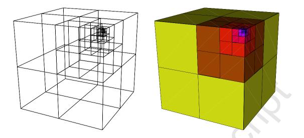
Figure 1: Example of a simple octree discretization of the unit cube. The unit cube is divided in 8 sub-cubes, which can be arbitrarily divided into 8 sub-sub-cubes, and so on. The sub-cubes that remain undivided at the end of the construction of the octree are called leaves which are used here as finite elements with which the partial differential equations are solved.
