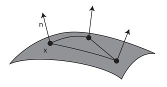
Figure 4: One of DOUAR's main feature is its ability to track interfaces. All interfaces are tracked through a set of particles defined by their coordinates  $\mathbf{x}$  and their normal to the interface  $\mathbf{n}$ . The particles are connected by triangles.
