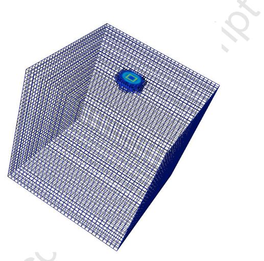
Figure 12: Final octree  $(L_u = 5, L_{max} = 9)$  generated by DOUAR for the square punch computations. Colour (from blue to red) indicates  $E'_2$
