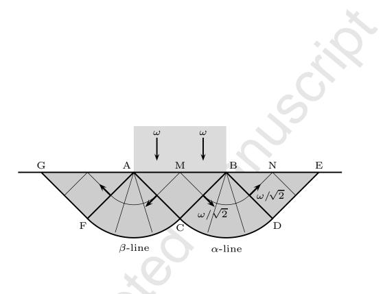
Figure 10: Prandtl's rigid-plastic solution. The indenter is shown in light grey while the material that has a non-zero velocity is shown in dark gray.  $\alpha$  and  $\beta$  slip lines intersect each other at  $\pi/2$  angles.
