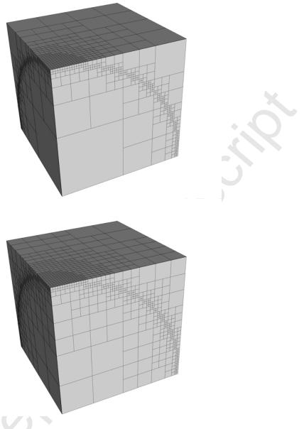
Figure 3: Example of an octree designed to represent a spherical shell of unit radius. The octree in the top panel has been constructed so that the region surrounding the shell is discretized with 'leaves' of level 6. The octree depicted in the bottom panel has been "smoothed", i.e. the condition that no two adjacent leaves (or elements) can vary in size by more than one level of octree division has been applied.
