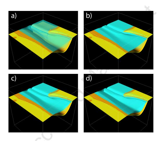
Figure 15: Final stratigraphy of the basin formed during the folding experiment described in Figure 14. a) The three stratigraphic markers are shown as semi-transparent cyan surfaces. b) to d) Each of the three stratigraphic markers is shown as an opaque cyan surface.
