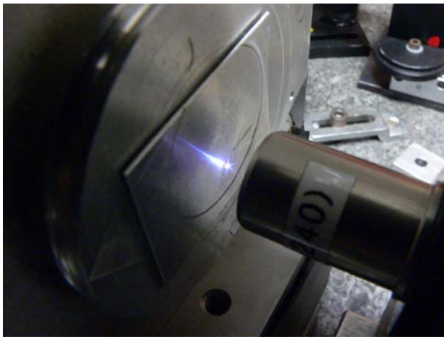
Fig. 7. (Color online) Photograph of the setup used for material processing. In this photograph the laser is focused 1 mm before the target to visualize the plasma in the air at the focused spot.
