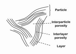
Figure 1. Schematic view of pores in clays. The stacking of clay layers forms particles containing interlayer pores ( $\leq$ nm). The aggregation of particles leaves empty regions referred to as interparticle pores (nm to  $\mu$ m). Interlayers can accomodate a few molecular layers of water, and the interparticle pores can be filled with an electrolyte solution, *i.e.* water and ions.
