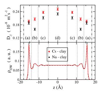
**Figure 4.** Water diffusion coefficient along the surfaces, as a function of distance to the surface (top), for Na<sup>+</sup> ( $\bullet$ ) and Cs<sup>+</sup> ( $\triangleleft$ ) counterions. Results are computed from the mean-square displacement of water molecules remaining in each of the region defined from the density profiles (bottom part of the figure).
