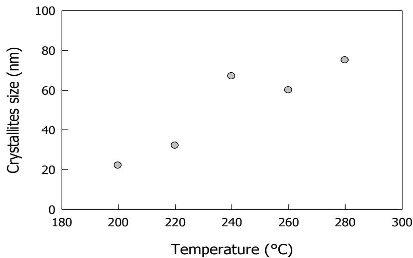
Figure 2. MOCVD of Cu from  $[\text{Cu}(\text{i-Pr-MeAMD})]_2$  on low carbon steel substrates. Estimation of particle size by X-ray diffraction line-broadening as a function of deposition temperature [14].
