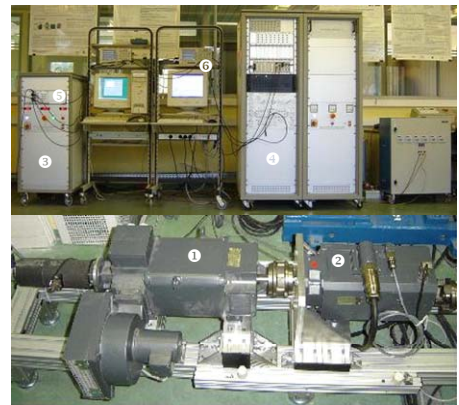
Fig. 13. Components of the G2ELAB test bench, Grenoble, France: ① DC motor, ② PMSG, ③ Power electronics for driving the DC motor, ④ Power electronics for driving the PMSG, ⑤ DSP TMS320F240 implementing DC motor control, ⑥ DSP DS1005 (dSPACE) implementing PMSG-based MCT control.
