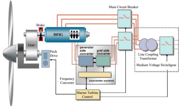
Fig. 5. Schematic diagram of a DFIG-based generation system.
