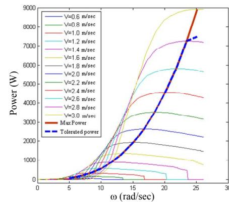
Fig. 7. Power curves for different tidal current speed.
