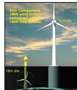
Fig. 4. Tidal turbine against an offshore wind turbine [© MCT].
