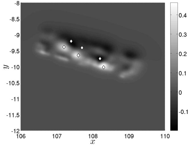
FIGURE 6. Location of the six numerical wave gauges (indicated by the symbol  $\diamond$ ) superposed with the steady state coseismic bottom displacement (only the vertical component in meters is represented here).
