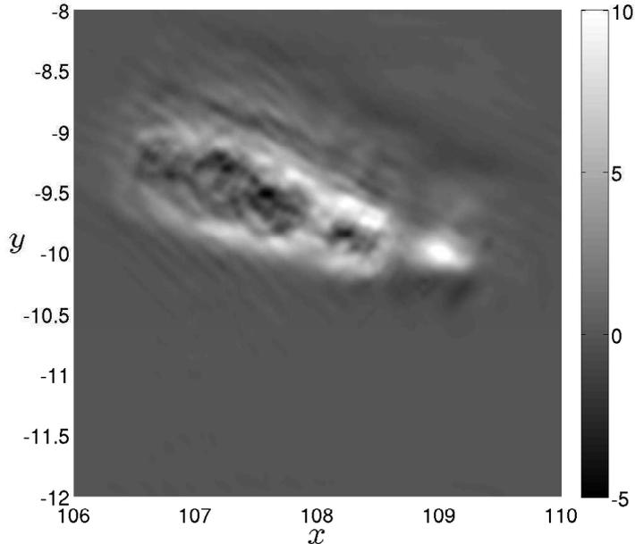
FIGURE 8. Relative difference between the free surface elevation at  $t_e = 220$  seconds computed according to the complete  $\eta_c(\vec{x}, t_e)$  (with horizontal displacements) and incomplete  $\eta_i(\vec{x}, t_e)$  (only vertical component) tsunami generation scenarios. The bottom moves according to the trigonometric scenario (2.1). The vertical scale is given in percents of the maximum amplitude of the incomplete scenario —  $\max_{\vec{x}} \eta_i(\vec{x}, t_e)$ .
