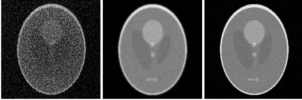
Figure 7: Noisy data, 360 detectors. Left: filtered back-projection solution. Center: time reversal solution. Right: control approach solution.
