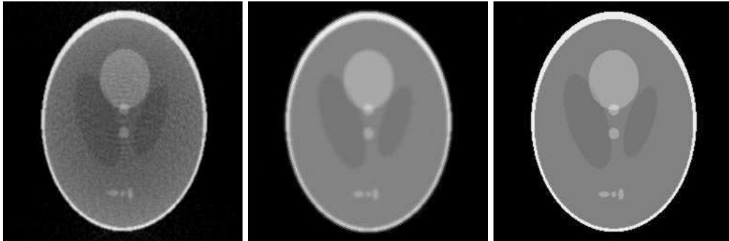
Figure 5: Noiseless data, 360 detectors. Left: filtered back-projection solution. Center: time reversal solution. Right: control approach solution.
