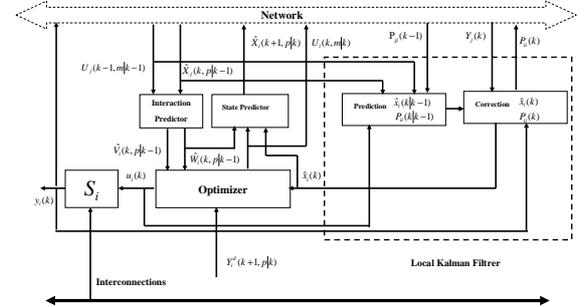
Fig. 2. Internal structure of the  $i$ th MPC sub-controller  $\mathcal{E}_i$ .
