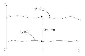
Figure 1: Domain considered for the Fowler model: h is the depth water,  $\eta$  the free surface and u the sandy bottom.
