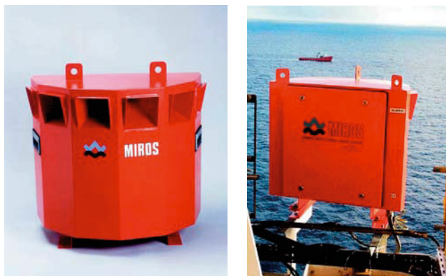
Figure 5.11: Left: The Doppler wave radar MIROS seen from the front with six horn antennas. The unit is 0.83 m wide and 0.89 m high. Right: The Doppler radar mounted on a platform in the North Sea.
