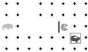
Figure 9. The robot sees a bison (animal V) and hears a crocodile (animal A). The robot will redirect its look immediately towards the crocodile.
