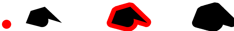
Fig. 3.28 Illustration of shape offsetting. Starting from the black set A and the red ball B (left), \delta_B A is constructed (middle and right.)
