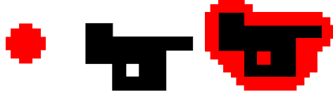
Fig. 2.20 Discrete dilation of the black shape S_d by the red kernel B_d .
