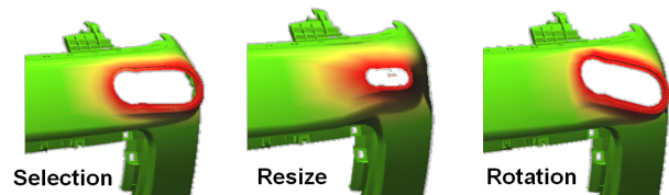
Figure 6: Deformation on dashboard ventilation outlet.
