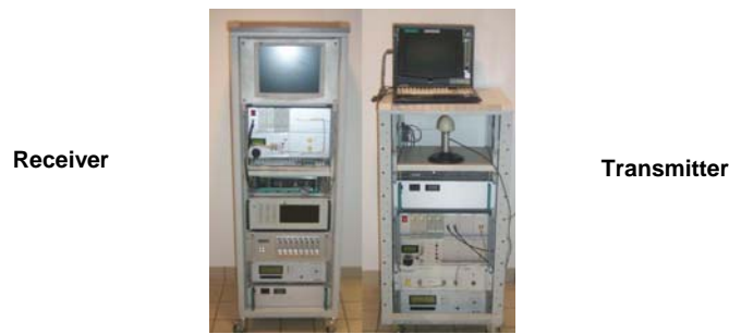
Fig. 2. MIMO channel sounder.
