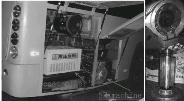
Fig. 16. A 50-kW switched reluctance motor in an experimental HEV bus" [31].
