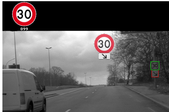
Figure 2. Illustration of detection and recognition of “arrow-type” supplementary sub-sign; note that proper handling of such sub-signs is essential for deducing actual speed limit, as they specify to which lane the speed limit of the traffic sign applies; other critical sub-sign include those for vehicle-specific or weather-specific speed-limits.
