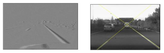
**Figure 4.** Lane-detection by Hough transform applied to gradient image; lane-changes are detected by analysis of lateral evolution of lanes in a memory of lane positions
