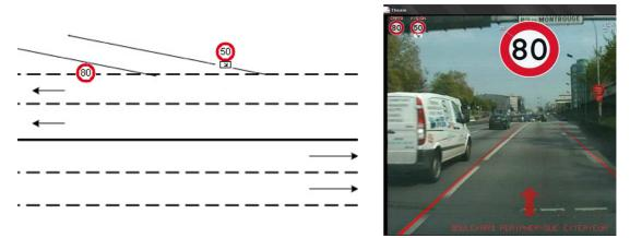
**Figure 3.** Left, an example in which both cartography and vision may provide the same wrong answer, when exiting; on the right, the decision between the 80 from cartography and the 50 from vision is more easily made by temporal logic than by some plausibility-based fusion of the 2 informations.
