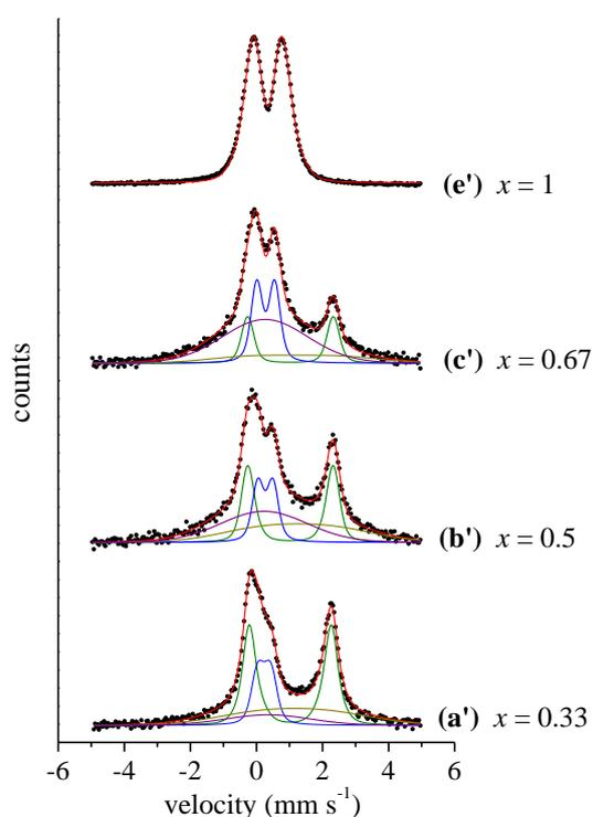
**Figure 2.** Backscattered Mössbauer spectra of  $\text{GR}(\text{CO}_3^{2-})$  at  $x = 0.33$  and  $\text{GR}(\text{CO}_3^{2-})^*$  oxidised at different values of the ferric molar fraction  $x$ . The spectra are recorded with method (i) at room temperature.
