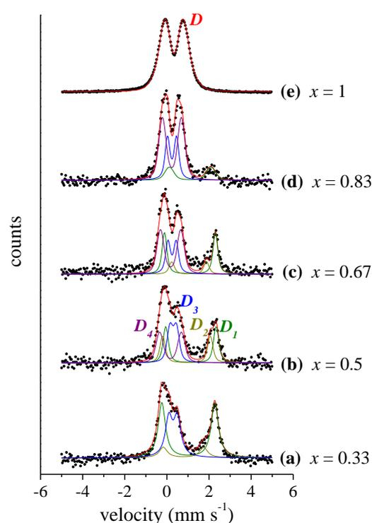
**Figure 3.** Backscattered Mössbauer spectra of  $\text{GR}(\text{CO}_3^{2-})$  at  $x = 0.33$  and  $\text{GR}(\text{CO}_3^{2-})^*$  oxidised at different values of the ferric molar fraction  $x$ . The spectra are recorded with method (ii) at room temperature.
