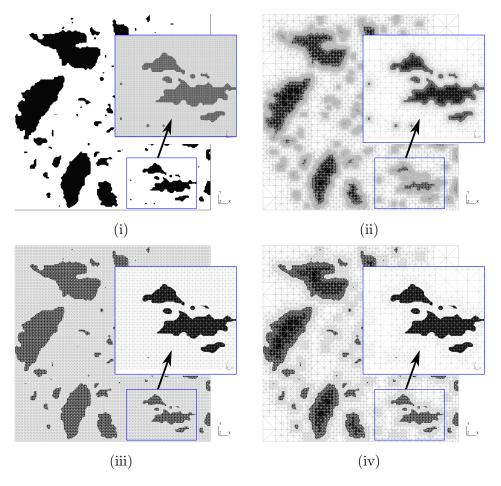
Figure 12: Comparison between uniform derefinment and octree derefinment (metallic-ceramic composite) ((i): the mesh has been omitted for clarity)
