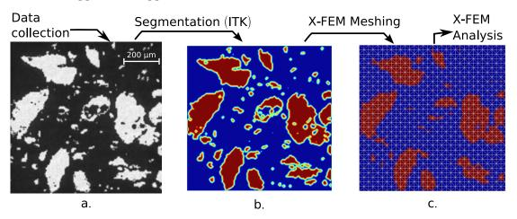
Figure 1: Numerical algorithm: a. data collection (reproduction of SEM sample of metallic composite - 24% TiC/stellite). b. segmentation using a Level set threshold based segmentation filter, and c. X-FEM computational mesh constructed incorporating the Level set data in enriched elements. (Image from [75])
