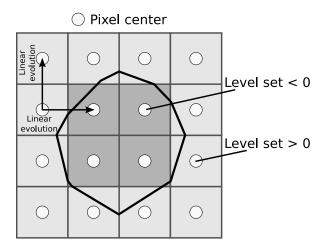
Figure 4: Subpixel precision of the location of the iso-zero
