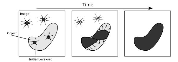
Figure 2: Segmentation process: a user-defined level set is evolved based on image features.
