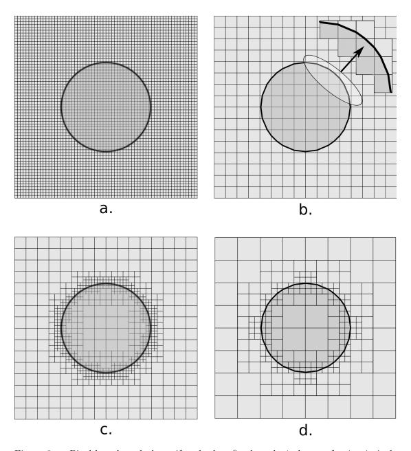
Figure 6: a. Pixel-based mesh; b. uniformly de-refined mesh, 1 element for  $4 \times 4$  pixels (note the degradation of the geometry); c. Octree mesh with maximum geometrical accuracy near the interface (1 element for 1 pixel); d. Octree with coarse accuracy near the interface (1 element for  $2 \times 2$  pixels here).
