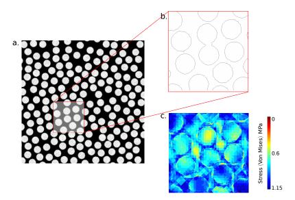
Figure 9: a. Idealized representation of the fiber-reinforced composite ( $512 \times 512$  pixels); b. Iso-zero of the Level set (material interface) for a sub-region ( $128 \times 128$  pixels); c. Von Mises stresses corresponding to the shearing micro-mode (mesh size  $2 \times 64^2$  elements).
