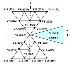
Fig. 3. Synthesized voltage vectors obtained using DSVM technique.
