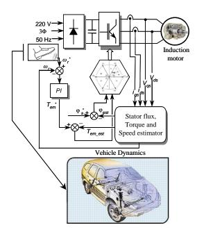
Fig.1. Basic direct torque control scheme.
