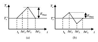
Fig. 5. Comparison of torque waveforms in one sampling period when  $C_T$  is 0: (a) Applying "3Z3", (b) Applying (33Z).
