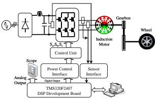
Fig. 6. The experimental setup.
