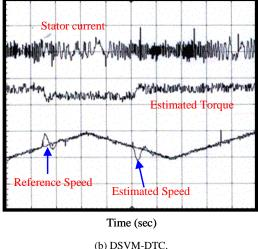
Fig. 7. Experimental performances of the proposed control approach.
