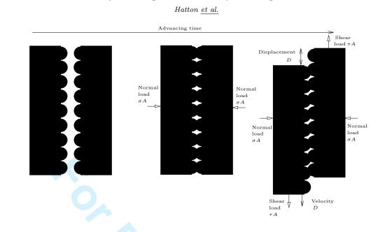
Figure 1. Schematic of sliding process involved in internal friction, with definitions of relevant quantities. A is cross-sectional area of facing surfaces.
