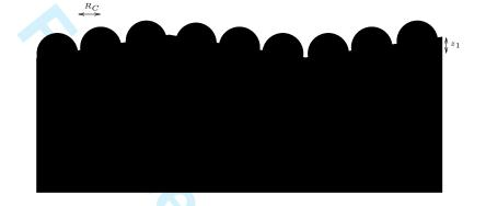
Figure 3. Schematic of surface topography with top-hat distribution of peak heights
