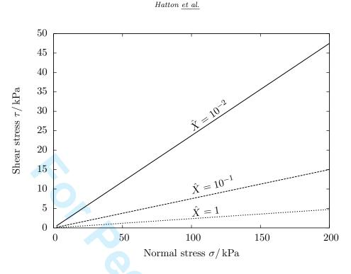
Figure 13. Sliding shear stress as function of normal stress. Three curves shown, corresponding to different values of dimensionless melt-water expulsion displacement  $\hat{X}$ . Other adjustable parameters fixed: dimensionless contact-breakage displacement  $\hat{Y} = 10^{-1}$ , dimensionless shear layer thickness  $\hat{Z} = 10^{-1/2}$ , asperity normal strain  $\epsilon_* = 8 \times 10^{-2}$ . Sliding velocity fixed:  $\dot{D} = 5.4563 \text{ mm/s}$ .
