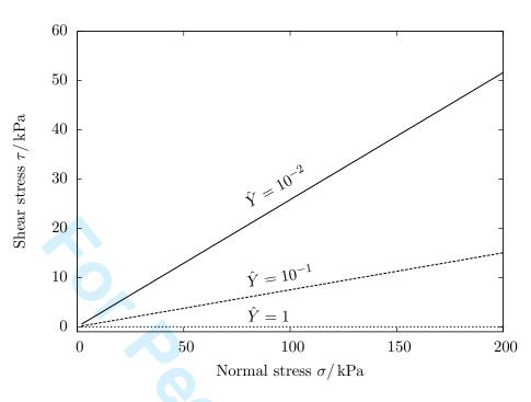
Figure 14. Sliding shear stress as function of normal stress. Three curves shown, corresponding to different values of dimensionless contact-breakage displacement  $\hat{Y}$ . Other adjustable parameters fixed: dimensionless melt-water expulsion displacement  $\hat{X} = 10^{-1}$ , dimensionless shear layer thickness  $\hat{Z} = 10^{-1/2}$ , asperity normal strain  $\epsilon_* = 8 \times 10^{-2}$ . Sliding velocity fixed:  $\dot{D} = 5.4563 \text{ mm/s}$ .
