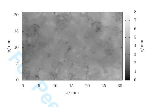
Figure 10. Topographic profile of an ice surface, which had undergone repeated back-and-forth sliding.
