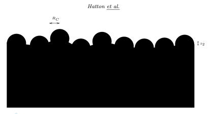
Figure 4. Schematic of surface topography with exponential distribution of peak heights
