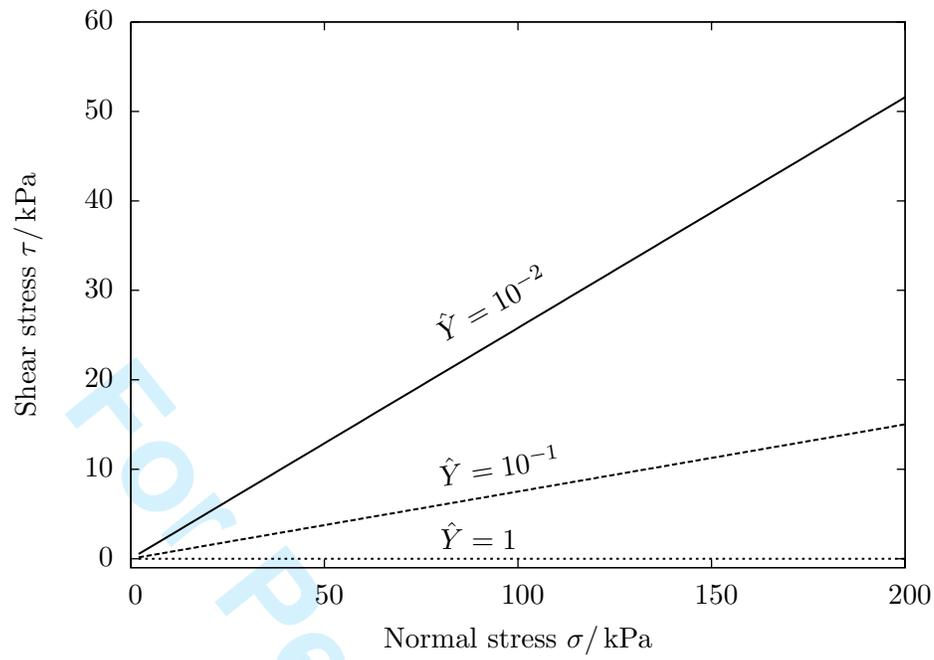
Figure 14. Sliding shear stress as function of normal stress. Three curves shown, corresponding to different values of dimensionless contact-breakage displacement  $\hat{Y}$ . Other adjustable parameters fixed: dimensionless melt-water expulsion displacement  $\hat{X} = 10^{-1}$ , dimensionless shear layer thickness  $\hat{Z} = 10^{-1/2}$ , asperity normal strain  $\epsilon_* = 8 \times 10^{-2}$ . Sliding velocity fixed:  $\hat{D} = 5.4563$  mm/s.
