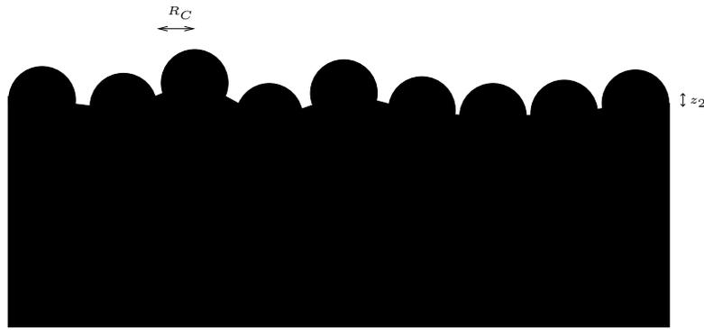
Figure 4. Schematic of surface topography with exponential distribution of peak heights
