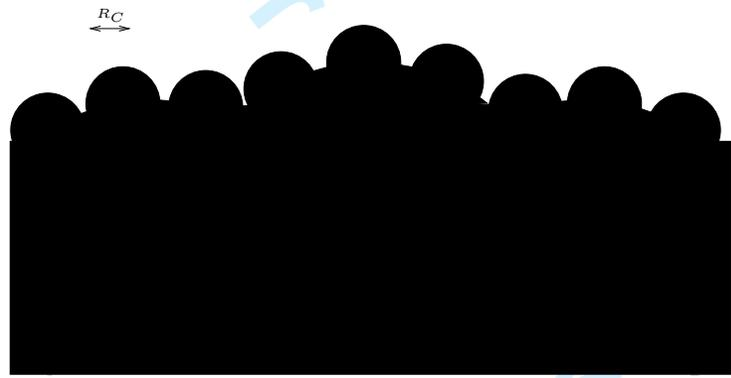
Figure 7. Schematic of two-step fractal surface topography.
