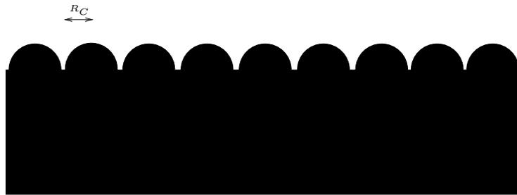
Figure 2. Schematic of surface topography with delta-function distribution of peak heights
