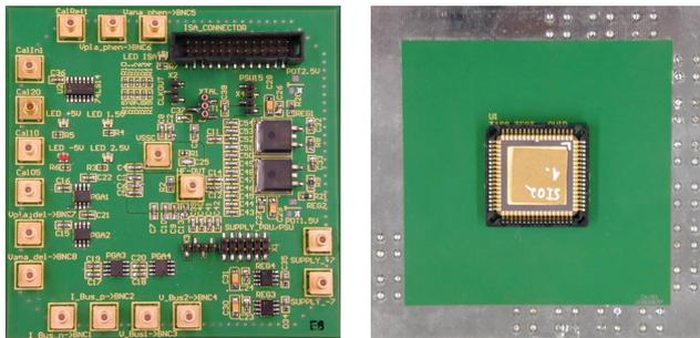
Figure 13: Top (left) and bottom (right) side of the TASC test board
