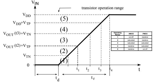
Figure 3: Transistor operation ranges during one switching phase
