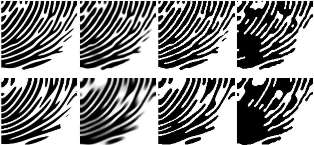
FIGURE 7. Various implementations of the affine curvature motion. the original image is displayed alone in the left column. In the other columns, from left to right: LLAS, FDS and FDS-stack filter at renormalized scales l = 4 (top) and l = 8 (bottom). In the case of the affine curvature scale space, the gradient amplitude keeps down ridge diffusion, unlike the mean curvature scale space. In general the affine smoothing performs better than the curvature motion (compare with Figure 8).
