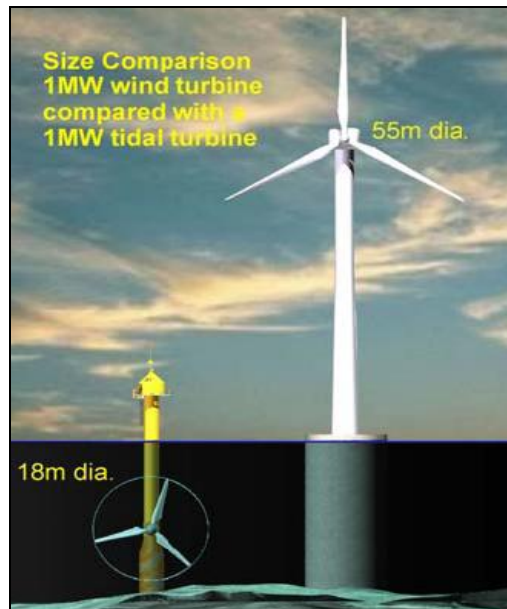
Fig. 4. Tidal turbine against an offshore wind turbine [© MCT].
