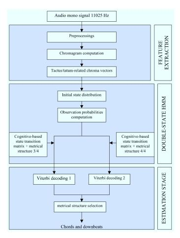
Fig. 1. General flowchart of the proposed model for simultaneous chord progression and downbeat estimation.
