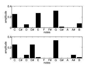
Fig. 3. Chord templates  $CT_1$  (top) and  $CT_{13}$  (bottom) for C Major and C minor chords considering 6 harmonics in the model.
