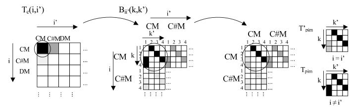
Fig. 6. In this figure, the darker the color, the higher the value in the transition matrix. The figures indicate: the chord transition matrix for a single-state HMM [left], the transition matrices for major to major chords in the case of double-states HMM, without taking into account the pim of the chord in the measure [middle left] and taking into account the pim of the chord [middle right] (lower value on transition pim3-pim1, pim4-pim1) and the pim transition matrices [right].
