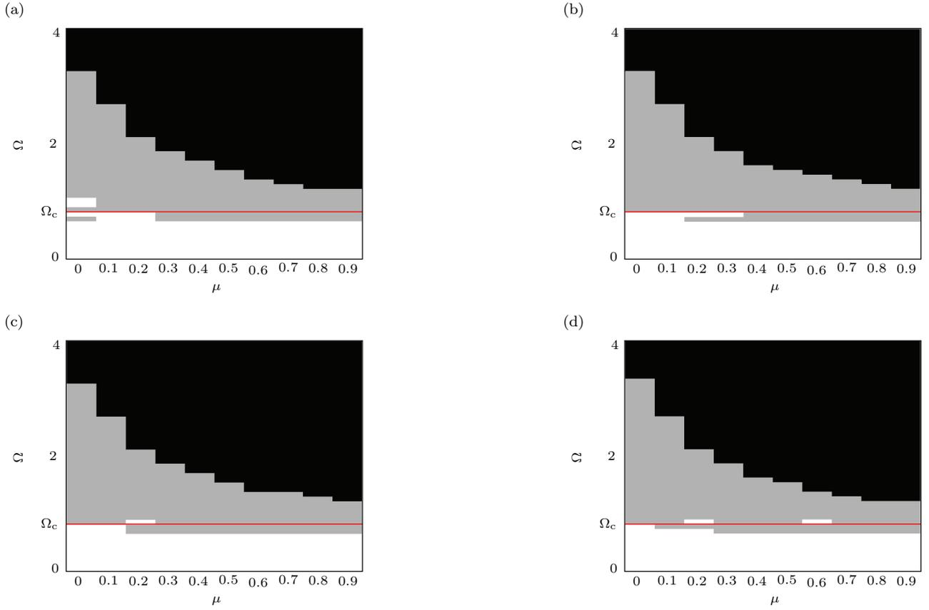
Figure 16: Motions detected with respect to  $\mu$  and  $\Omega$  with the CM reduced order model: divergent motions (■); locked motions (■) and damped motions (□): (a)  $\phi = 22$ ; (b)  $\phi = 44$ ; (c)  $\phi = 66$ ; (d)  $\phi = 88$ .
