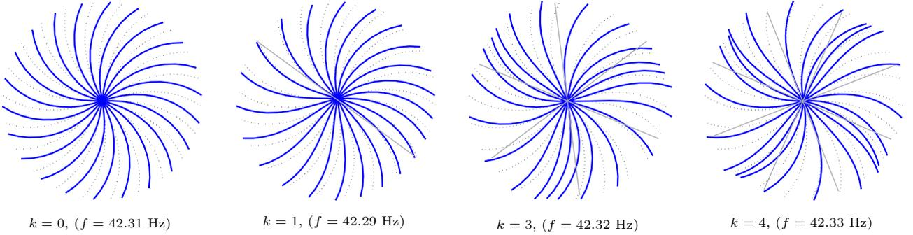
Figure 3: First vibration modes of the bladed disk
