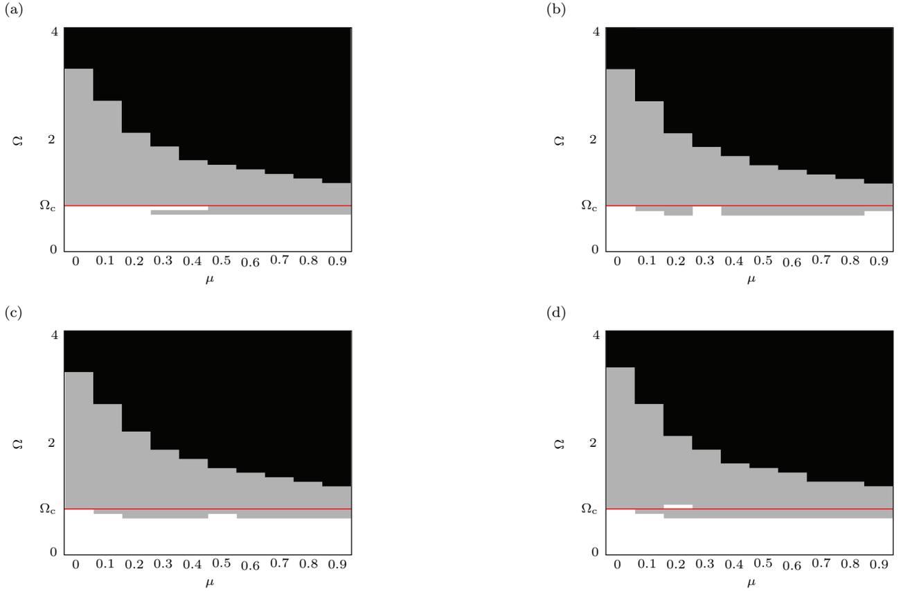
Figure 15: Motions detected with respect to  $\mu$  and  $\Omega$  with the CB reduced order model: divergent motions (■); locked motions (■) and damped motions (□): (a)  $\eta = 22$ ; (b)  $\eta = 44$ ; (c)  $\eta = 66$ ; (d)  $\eta = 88$ .
