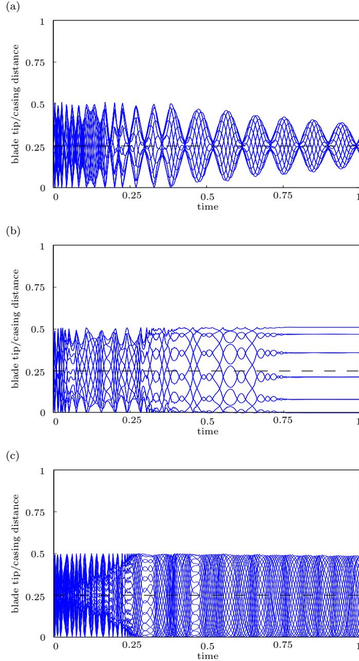
Figure 9: Blade tip/casing distances, initial clearance (-----). (a) damped motion:  $\Omega = 0.4$ ,  $k = 2$ ; (b) locked motion:  $\Omega = 0.96$ ,  $k = 2$ ; (c) sustained motion:  $\Omega = 1.68$ ,  $k = 3$ .
