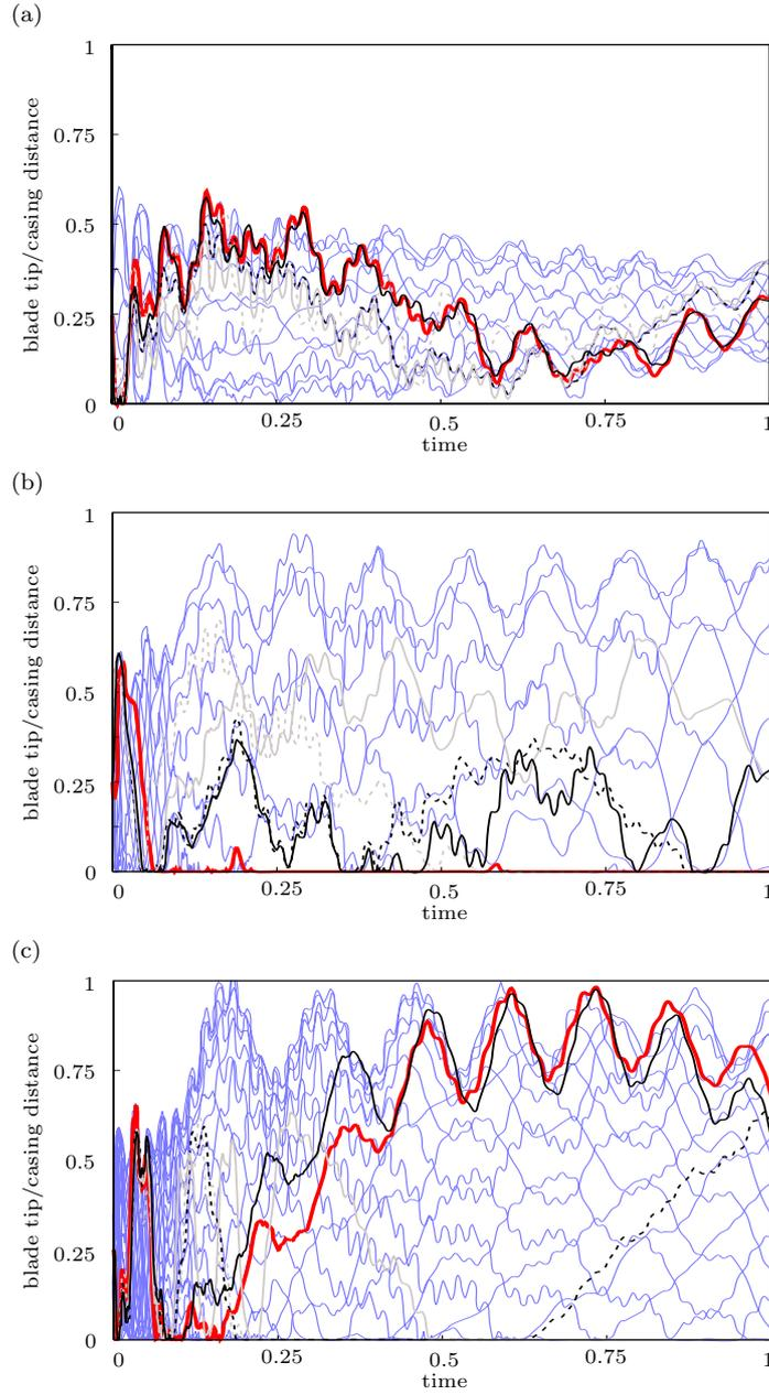
Figure 13: Convergence of the results obtained with CM method  $\phi = 0$  (---);  $\phi = 44$  (-.-.-);  $\phi = 88$  (—);  $\phi = 220$  (—);  $u_{fe}(t)$  (—). (a) damped motion, blade 10,  $\Omega = 0.56$ ,  $k = 2$ ; (b) locked motion, blade 9,  $\Omega = 1.12$ ,  $k = 2$ ; (c) sustained motion, blade 2,  $\Omega = 1.28$ ,  $k = 3$ .
