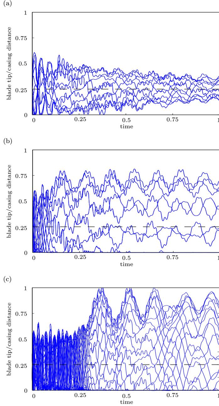
Figure 11: Blade tip/casing distance for the interaction motions detected, initial clearance (.....). (a) damped motion :  $\Omega = 1.2$  ( $k=2$ ); (b) locked motion :  $\Omega = 1.56$  ( $k=2$ ); (c) sustained motion :  $\Omega = 1.38$  ( $k=3$ ).
