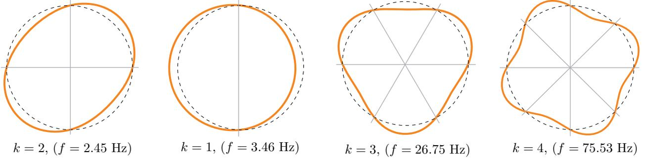
Figure 5: First vibration modes of the casing
