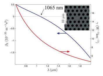
Fig. 2. Dispersion curve for the fundamental mode exhibiting a zero-dispersion wavelength at 1065 nm and nonlinear coefficient as a function of the wavelength. The inner plot shows a SEM image of the microstructured fiber cross-section.
