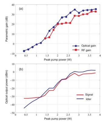
Fig. 6. (a) Net parametric gains with respect to the pump power. Circle dot (blue): parametric gains calculated with powers of the signal from optical spectra. Square dot (red): parametric gains calculated with RF signal outputs from the PD. (b) Optical output power of the signal (blue curve) and the idler (red curve).
