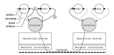
Fig. 1. Airplug architecture, intra- (1) and inter- (2) vehicle communications.
