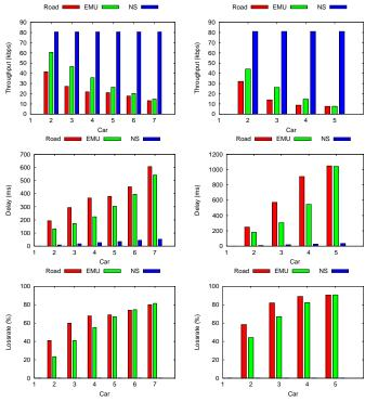
Fig. 5. Comparisons of road tests, EMU and ns-2 with average inputs for EMU. On the left, a stopped convoy of 7 vehicles. On the right, a moving convoy of 5 vehicles. From top to bottom: throughput, delay, loss-rate.
