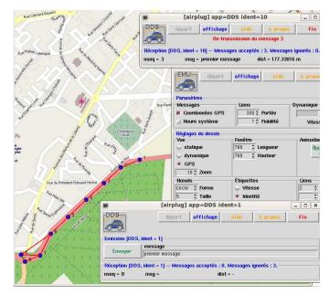
Fig. 3. Emulation of the DDS application on a convoy of 9 vehicles generated by the GPS application from a real GPS trajectory obtained on road N131, Compiègne, France. We can see the DDS applications running on vehicles 1 and 10, as well as parameters of EMU. Maps by *OpenStreetMap.org*.
