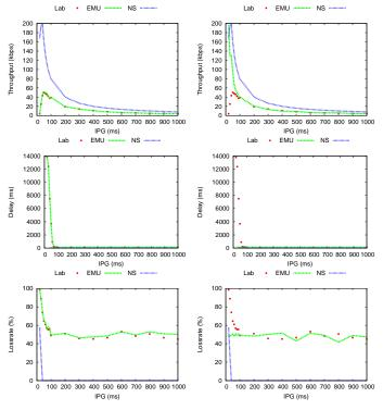
Fig. 4. Comparisons of in-lab tests, EMU and ns-2 depending on the interpacket gap (IPG) in milliseconds. On the left, accurate inputs for EMU. On the right, average inputs. From top to bottom: throughput, delay, loss-rate.
