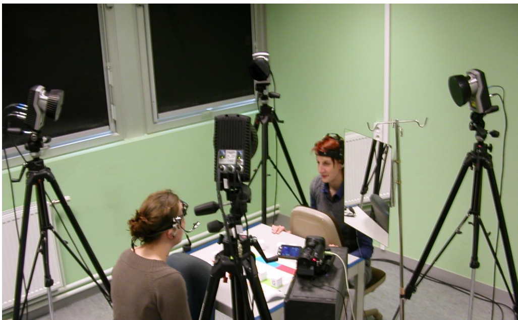
Figure 2 - Technical setup of the experiment comprising head mounted eye tracking, head mounted microphones, video recording, and motion capture of head movements.
