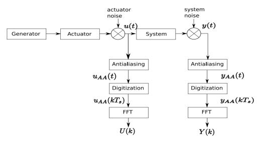
Figure 1: FRF measurement (adapted from [20]).
