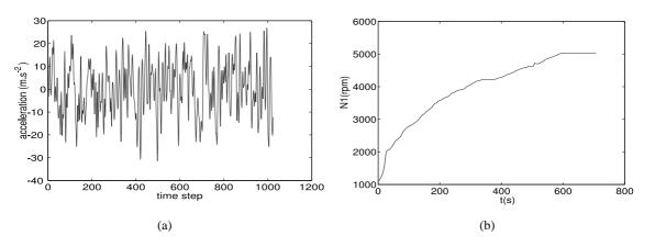
Figure 3: (a) Raw accelerometric data; (b) LP shaft angular velocity in rpm.
