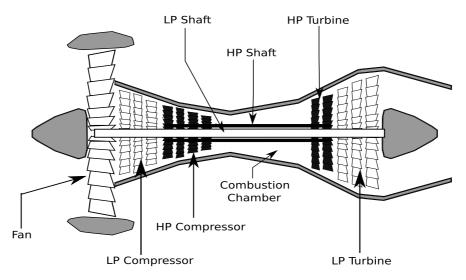
Figure 2: Turbofan engine. Simplified diagram of fan, low-pressure and high-pressure compressors and turbines attached to their respective shafts.
