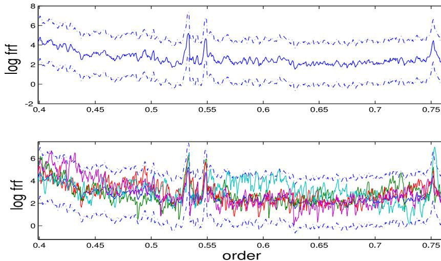
Figure 4: FRF in the order domain (top) predicted mean and associated confidence interval (bottom) superimposed FRF of all engines.
