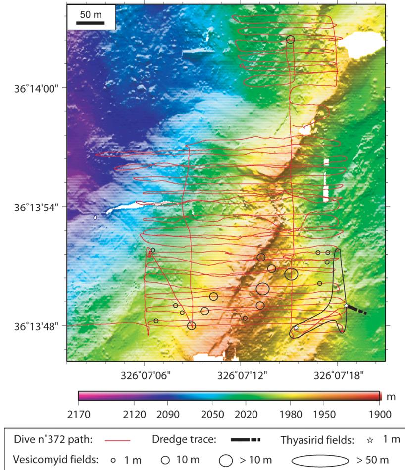
**Figure 2.** High resolution multibeam bathymetry acquired by ROV Victor at an altitude of 50 m in the “Clamstone” area (background). The red line shows the track of Dive 372, performed at low altitude, in order to ensure full coverage of vertical OTUS photographs (see Figures 1 and 5). The distribution of fossil bivalve fields is shown by ellipses and stars.
