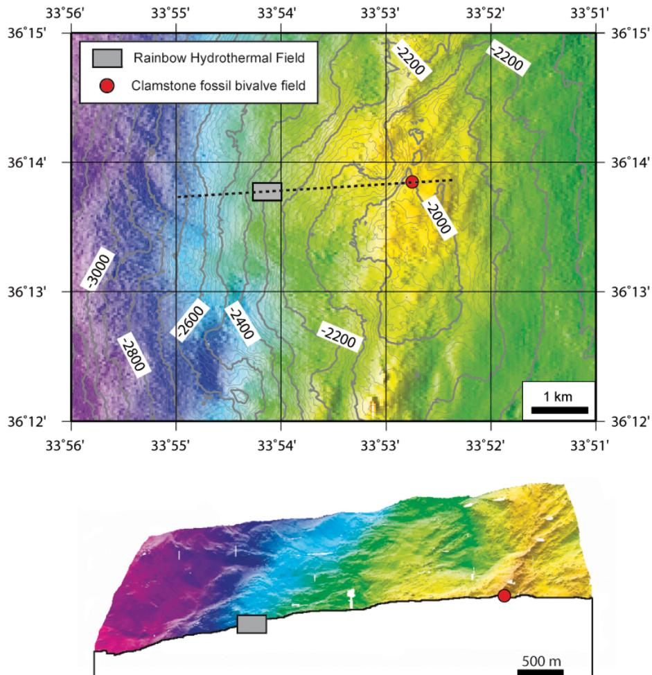
**Figure 1.** (top) Shipborne multibeam bathymetry on Rainbow Massif (cruise Flores of the R/V *L'Atalante*), and (bottom) the perspective view from high resolution multibeam bathymetry acquired by ROV Victor at an altitude of 50 m (adapted from *Dyment et al.* [2009]), showing the location of the hydrothermal site Rainbow and the “Clamstone” fossil bivalve fields.
