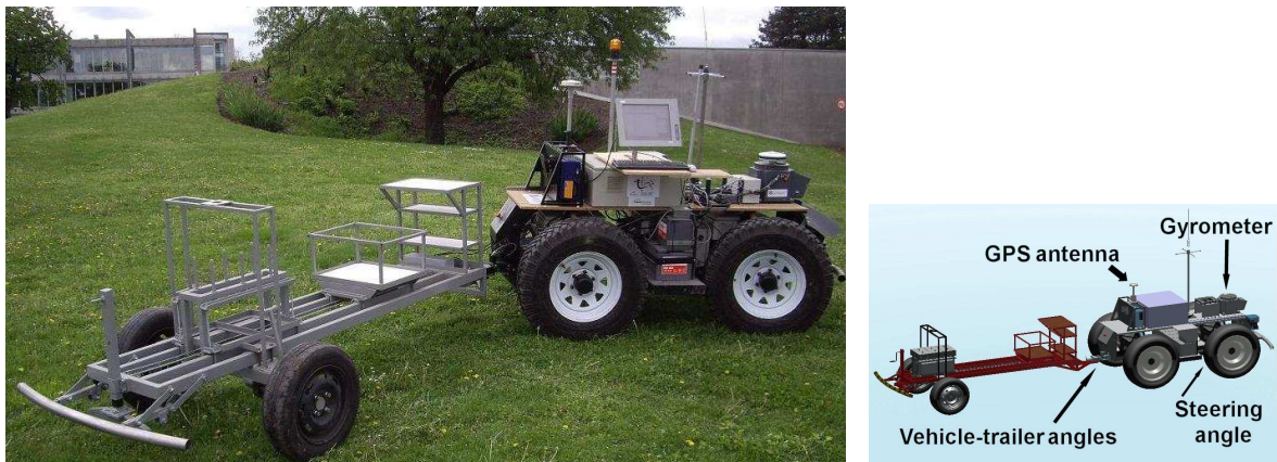
Fig 8: Experimental vehicle-trailer system
