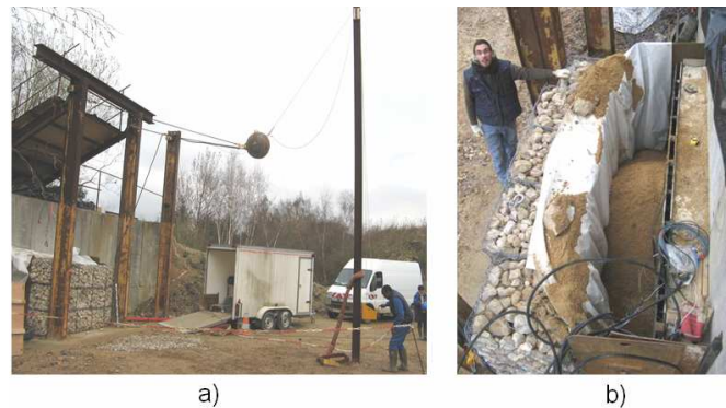
Figure.2. Overview of the experimental device (a) and the impacted structure during the implementation (b).
