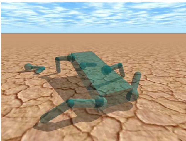
Fig. 1. An hexapode with two lost legs: how could we make a control system adaptive to such a situation ?
