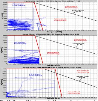
walking gait, the values of the torques (12 Nm at the hip, 8 Nm at knee and ankle) are sufficient.
