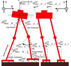
Fig. 3. Extreme angles characterizing ROBIAN Locomotion
