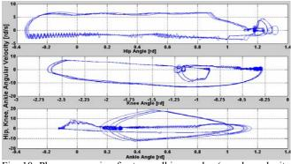
Fig. 10. Phase succession for ten walking cycles (angular velocity of Hip, Knee and ankle function of their corresponding angle
