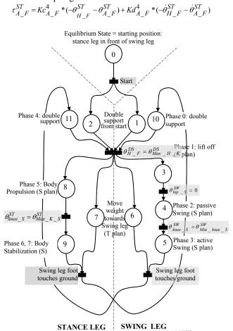
Fig. 4. Petri Net Algorithm for Robian Dynamic Walk (S\_Plan or Sagital Plan, F\_Plan or Frontal Plan)
