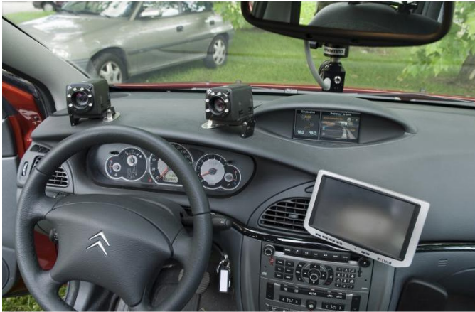
Figure 6. Driver interface: active gas pedal, audio and screen display. The two cameras on the dashboard are used for eye-tracking.
