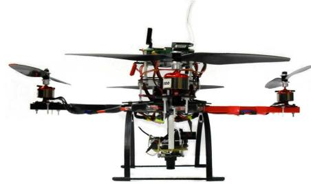
Fig. 3. Four rotor helicopter with a camera
