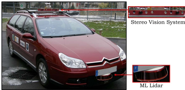
Figure 3. The experimental vehicle with the stereo vision system and the IBEO Alasca XT
