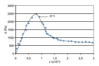
**Figure 3.** Uniaxial stress/strain diagram at temperature  $T = 20^{\circ}C$  and  $\dot{\varepsilon} = 10^{-2}s^{-1}$  showing the mechanical properties of the model material slope 1.
