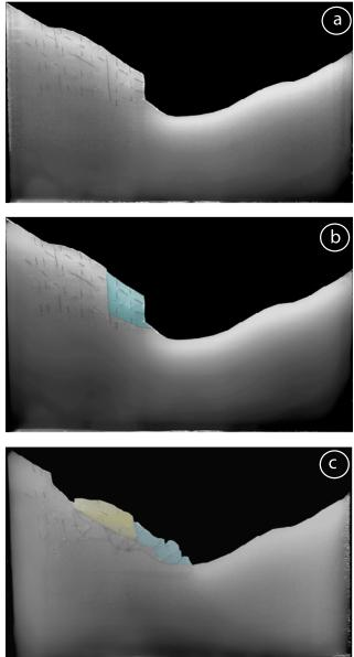
**Figure 6.** Experiment 3. (a) Initial highly prefractured model with some continuous joints. In this case the fractures assume to have initiated the two Randa rockslides are longer than any others. (b) Cross section realized at an early stage of evolution (after 100 acceleration stages). The first block is in blue and the second one in yellow. (c) Cross section realized at an advanced stage of evolution (after 120 acceleration stages).
