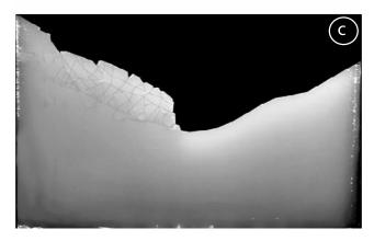
**Figure 5.** Experiment 2. (a) Initial highly prefractured model with discontinuous same length joints, (b) cross section realized at an early stage of evolution (after 100 acceleration stages), and (c) cross section realized at an advanced stage of evolution (after 120 acceleration stages).
