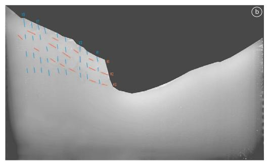
**Figure 2.** (a) View from above of the rigid box containing the model  $(0.14 \times 0.14 \text{ m in section})$ . This box is located on the mobile platform of the vertical accelerator, and (b) cross section of the model corresponding to the west-east cross section of the Grossgufer hillside. Vertical discontinuous fractures have been numbered from V1 near the valley to V9 near the summit and the subhorizontal fractures from H3 for the deeper to H1 for the shallower.
