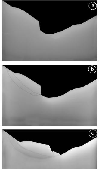
**Figure 4.** Experiment 1. (a) Initial homogeneous model, (b) cross section realized at an early stage of evolution (after 100 acceleration stages), and (c) cross section realized at an advanced stage of evolution (after 120 acceleration stages).
