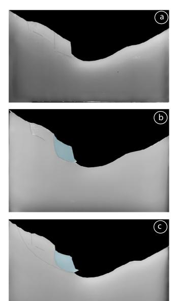
**Figure 7.** Experiment 4. (a) Initial slightly prefractured model, (b) cross section realized at an early stage of evolution (after 100 acceleration stages), and (c) cross section realized at an advanced stage of evolution (after 120 acceleration stages).
